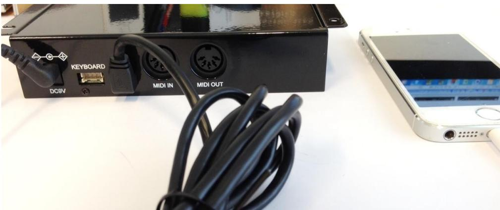
Now launch the app. The app should be launched only after the ProRecord has been calibrated, or otherwise your Apple device won't recognize it. Press "Load" in order to fully connect to the ProRecord. The Reverb setting should switch from "off" to "on" – this indicates that the connection works.
